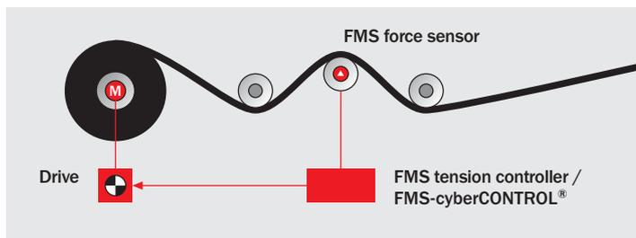
**FMS tension control system:** Force sensors determine the exact material tension and send a signal proportional to the tension to the FMS controller. FMS tension controllers process the signals from the force sensors and send the required correction value to the drive, brake or clutch.
